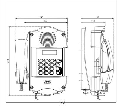
Explosion-proof EEx IIC IP66 telephone for wall mounting, outdoor, for the locale industrial and noisy P/N TLA 229 A
